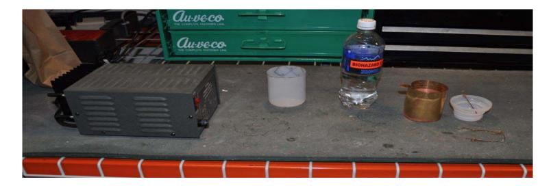
Solution: 650ml of water 1ml of 28% hydrochloric acid
