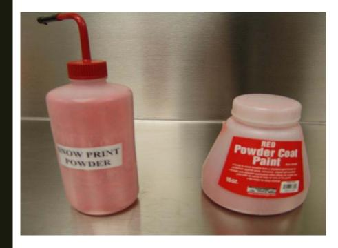
This works because powder coat paint is actually plastic. It will not combine with water and the powder is very fine. All we do is shake the bottle and squeeze out the powder that is in the air in the bottle. This results in a nice even thin coat of powder. This product works no matter how long it is in the cold and is not affected by varying storage temperatures (being in the car). The bottle picture here will last us years and cost \$6.00.
